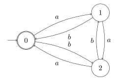
(The syntax used here defines initial states by an ingoing arrow (without a label), and final states have a double circle.)
